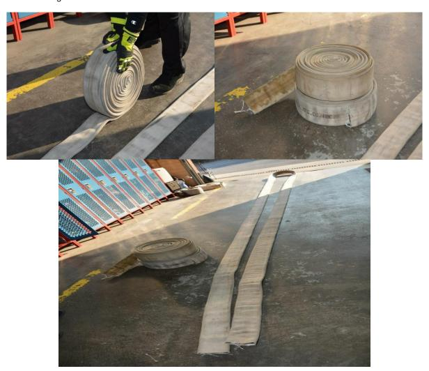
Re-roll two (2) of the sections of hose (coil). These coils will be used for the center of the ball. *Note: Re-roll the coils as tight as possible.*
