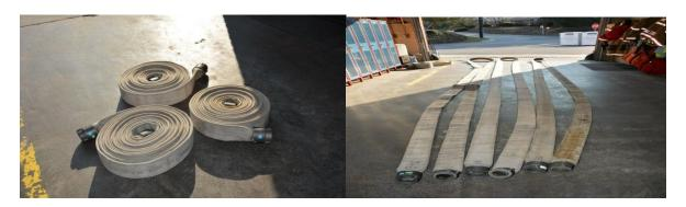
If the hose you are using still has the couplings, you will need to remove them. Unroll each section of hose, and line up the couplings as shown. Note: If the hose does not have couplings, leave two (2) rolls coiled up, and unroll one that will be used later.
