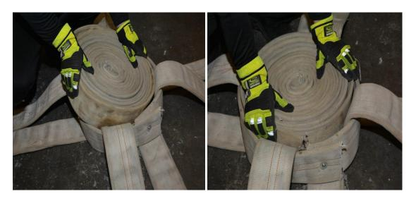
Once the coil is in the band, kneel on the coil and pull the weave straps tight.
