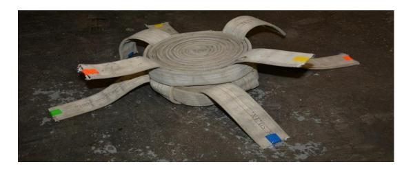
• Once the coil is in the band, kneel on the coil and pull the weave straps tight.
