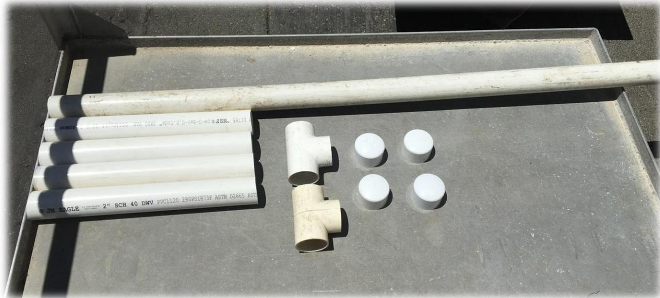
**STEP 2** Form the two “sides” of frame by gluing shorter PVC pipes to three-way connectors as shown below. Glue end caps on ONE end of each “side” tube.
