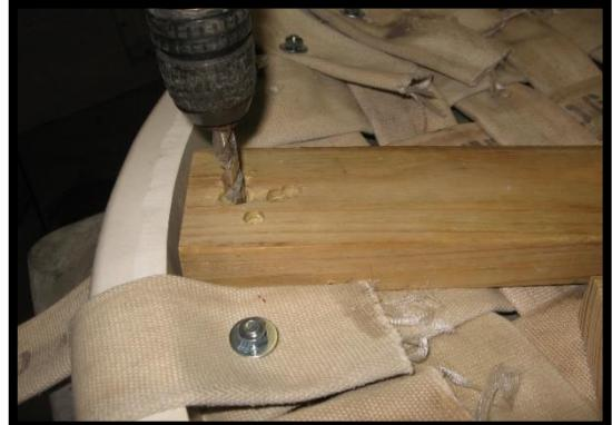
**STEP 7.** Secure each piece of fire hose with a nut, bolt, and two washers (a washer on each side to prevent the nuts and bolts from pulling through the fire hose). Repeat with each piece of fire hose. Pull the fire hose as tight as possible when securing the second end of a piece so that the hammock will be taut. When done, trim excess fire hose, leaving only about 2" past the nut and bolt.
