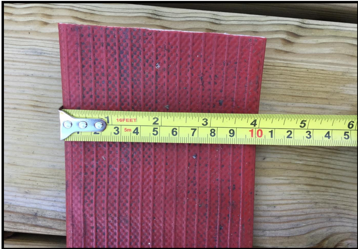
Fig. 2: Measuring the width of your fire hose.
