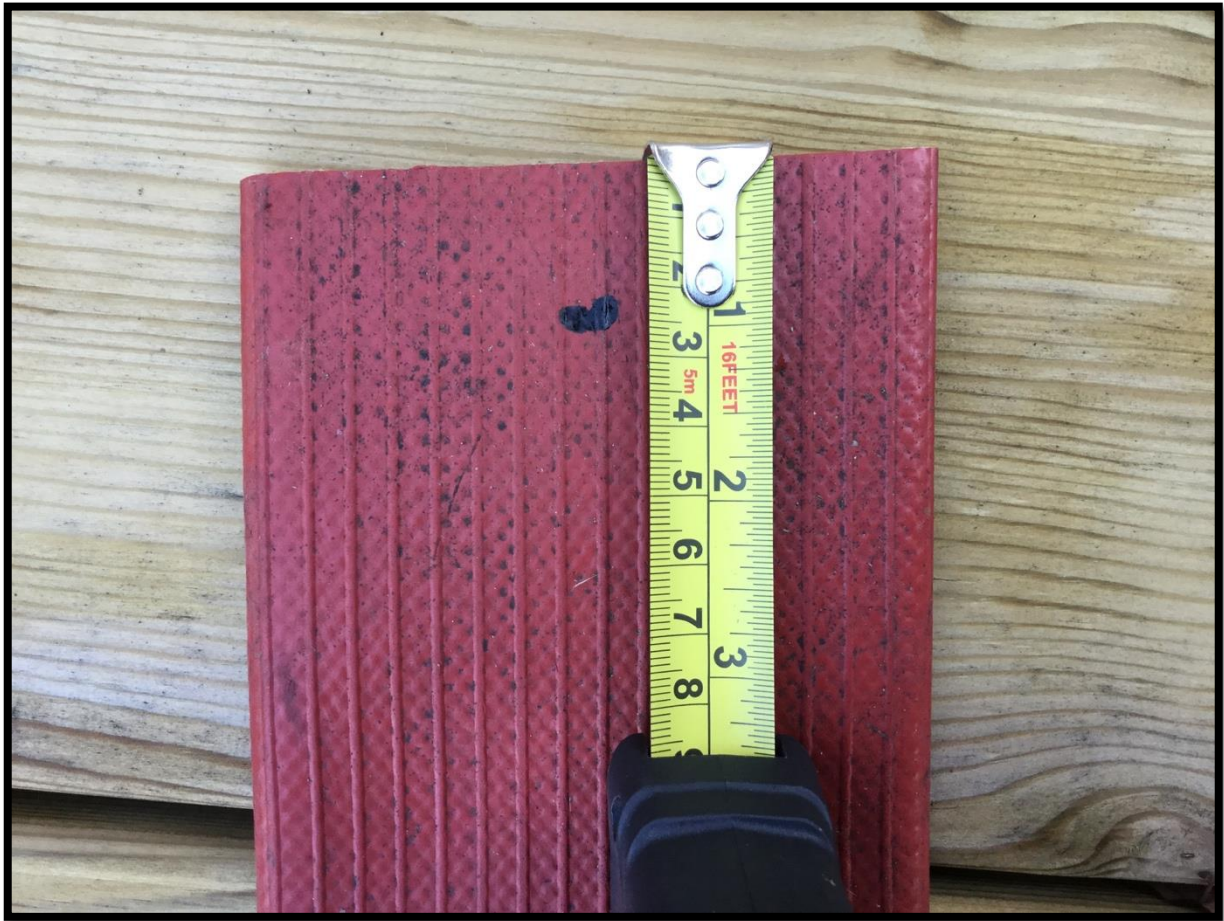
Fig. 4: Measuring and marking the holes to be drilled into the ends of the fire hose.
